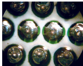
Solder paste and preforms reflowed
