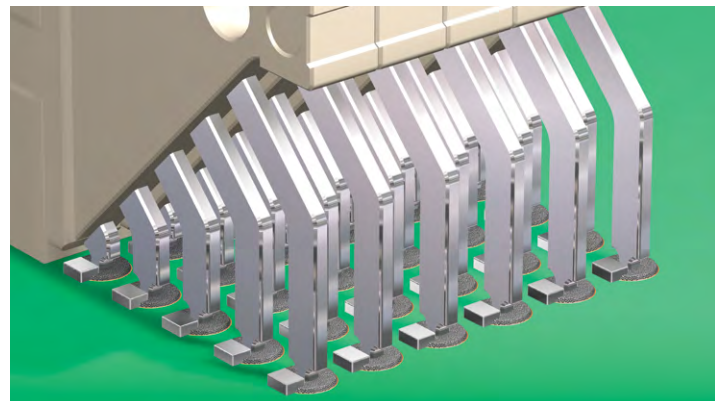
Solder paste and preforms reflowed
