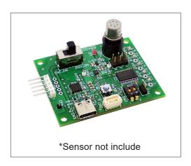
This module converts sensor output voltage into a five-level voltage output using the signal processing software to provide the Indoor Air Quality Level (VAQL) output. The LED equipped on the module changes color to indicate the Indoor Air Quality Level (VAQL).
