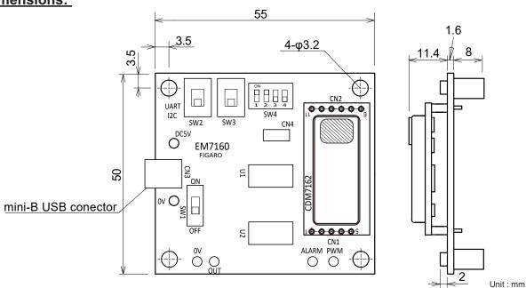
Note 1) Standard CDM7162 CO<sub>2</sub> sensor modules (without terminal pins) are available for additional purchase. To attach a standard CDM7162 to the evaluation module, terminal pins available in the marketplace should be soldered to the standard CDM7162.
